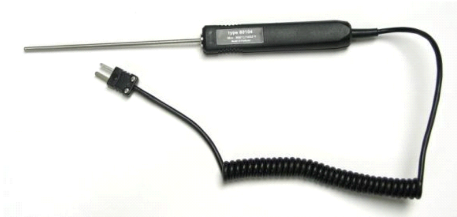
Type K Ni-CrNi. With spiral cord and insulating handle.
